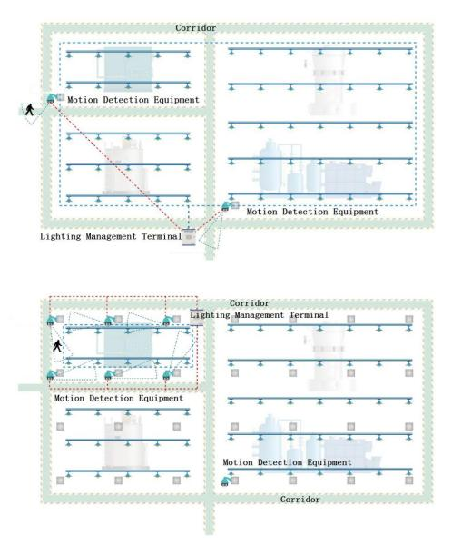
During the inspection process, the staff can be equipped with handheld devices to realize where the lights are on where the person walks.
