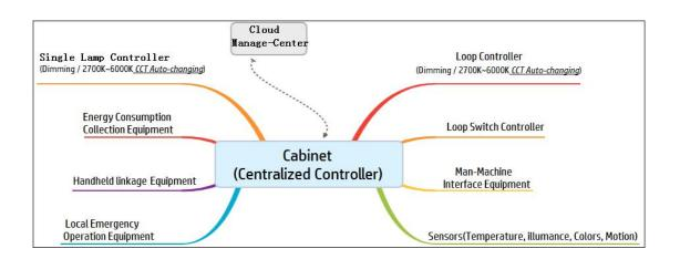
Generally speaking, the system are divided into cloud management center equipment, human-machine interface equipment, local management center equipment, lighting fixture control equipment, sensor equipment, and debugging equipment.
